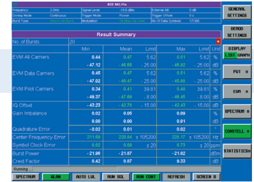
Fig. 2: Display of the main modulation parameters in the Result Summary: The measurement covering 20 bursts shows an EVM of -47.12 dB for the best burst (min. peak) and -45.92 dB for the worst burst (max. peak) as well as an average EVM of -46.55 dB for all bursts. Output power (with regard to burst) and crest factor are also displayed. Quick and easy determination, for example, of the EVM dependence on the output power of an amplifier is thus possible. The analyzer's auto level function allows it to follow level changes without manual setting or corrections.
