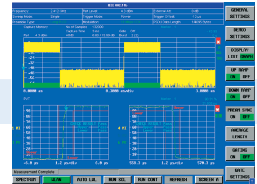
Fig. 5: Measurement of the rise and fall times for an IEEE 802.11b signal. Adjustable averaging ensures repeatable and stable results.
